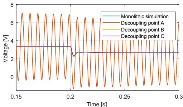
Fig. 12. Test case 2: time domain response of  $x_2$  with co-simulation interface of sampling periods of 0.05 ms and time delay of 0.5 ms
