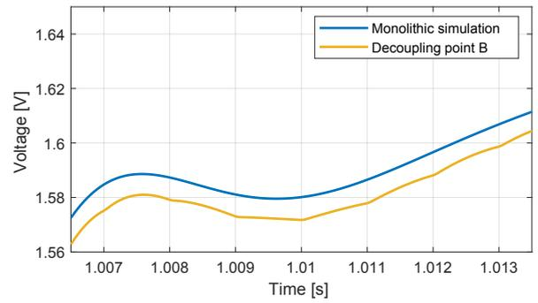
Fig. 8. Test case 1.1: time domain response of  $x_2$  with co-simulation interface of sampling period 1.0 ms, and time delay of 0.05 ms
