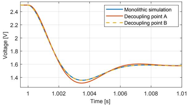
Fig. 6. Test case 1.1: time domain response of  $x_2$  with co-simulation interface of sampling period 0.05 ms, and time delay of 0.05 ms
