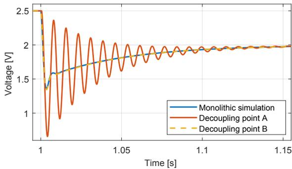
Fig. 7. Test case 1.1: time domain response of  $x_2$  with co-simulation interface of sampling period 0.05 ms, and time delay of 0.5 ms
