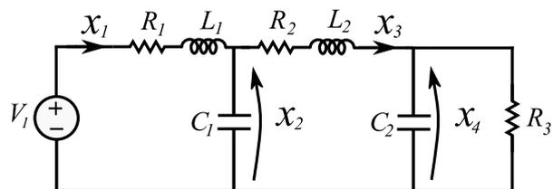
Fig. 11. Test Case 2 - simple electrical circuit
