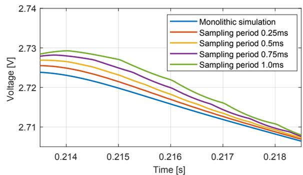
Fig. 13. Test case 2: time domain response of  $x_2$  with co-simulation interface of time delay of 0.05 ms and sampling periods of 0.25 ms, 0.5 ms, 0.75 ms, and 1.0 ms for decoupling point B
