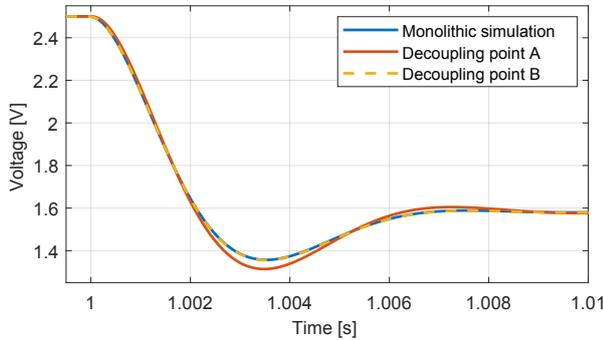
Fig. 6. Test case 1.1: time domain response of  $x_2$  with co-simulation interface of sampling period 0.05 ms, and time delay of 0.05 ms
