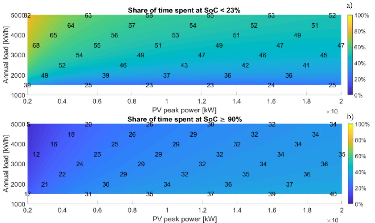
Figure 3: Overview of SoCs as a function of annual load and installed PV power. a) shows how much time was spent at SoCs below 23% (i.e. empty, as 22% are the lowest allowed value) and b) the amount of time spent at an SoC  $\geq$  90% (i.e. full).
