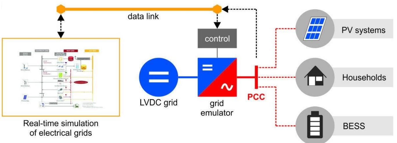
Figure 1: Schematic setup of the InFIS infrastructure. Real-time simulation of the electrical grids, PV generation and parts of household loads are simulated while the grid emulator, parts of household loads and the battery electric storage system (BESS) are implemented in hardware
