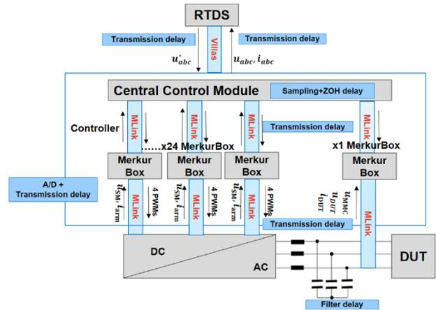
Figure 7: Structure of the communication of the grid emulator
