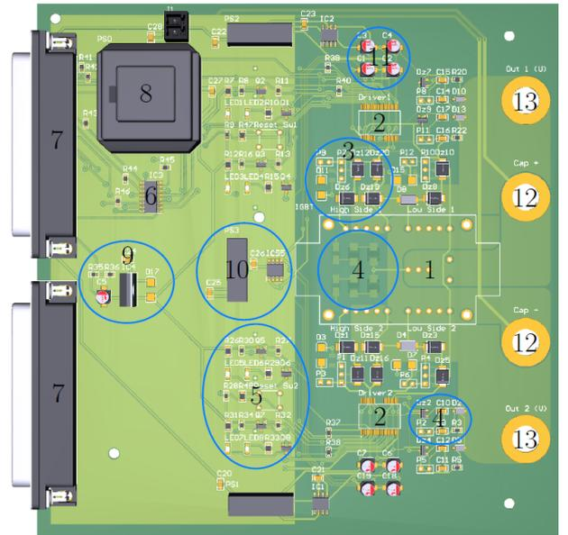
Figure 5: PCB of the auxiliary power supply circuit, the gate driver circuit and the IGBT modules (see Table 3 for details)
